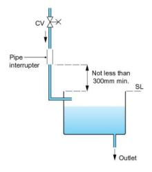
'Type DC – Pipe interrupter with permanent atmospheric vent' means a non-mechanical backflow prevention device with a permanent unrestricted air inlet, the device being installed so that the flow of water is in a vertical downward direction.
