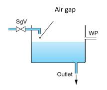
'Type AG – Air gap arrangement with minimum size circular overflow' means a non-mechanical backflow prevention arrangement of water fittings with an air gap; together with an overflow, the size of which is determined by measure or a vacuum test.
