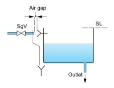
'Type AD – Air gap with injector' means a non-mechanical backflow prevention arrangement of water fittings with a horizontal injector and a physical air gap of 20 millimetres or twice the inlet diameter, whichever is the greater.
