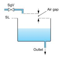
'Type AA – Air gap with unrestricted discharge' means a non-mechanical backflow prevention arrangement of water fittings where water is discharged through an air gap into a receptacle which has at all times an unrestricted spillover to the atmosphere.
