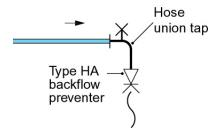
'Type HA – Hose union backflow preventer' means a mechanical backflow prevention device for fitting to the outlet of a hose union tap and consisting of a single check valve with air inlets that open if the flow of water ceases.
