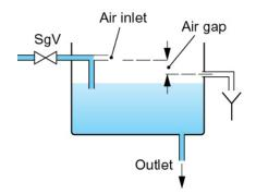
'Type AC – Air gap with vented submerged inlet and circular overflow' means a non-mechanical backflow prevention arrangement of water fittings with a vented, but submerged, inlet; the air gap being measured vertically downwards from the lowest point of the air inlet to the critical level.
