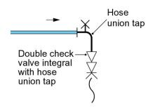
'Type HUK1 – Hose union tap incorporating a double check valve' means a hose union tap in which a verifiable double check valve has been incorporated into either the inlet or outlet of the tap.
