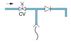
'Type HC – Diverter with automatic return' means a mechanical backflow prevention device used in bath/shower combination tap assemblies which automatically returns the bath outlet open to atmosphere if a vacuum occurs at the inlet to the device.
