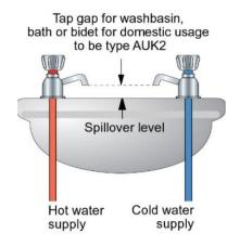
'Type AUK2 – Domestic tap gap' means the height of air gap between the lowest part of the outlet of a tap, combination fitting, shower head or other fitting discharging over a domestic sanitary appliance or other receptacle, and the spillover level of that appliance, where a fluid category 2 or 3 risk is present downstream.
